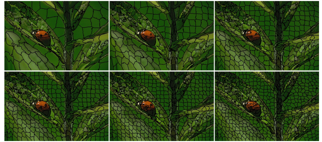
Fig. 1. Example DES results with different number of segmentations. From left to right, up to bottom: 100, 200, 300, 400, 500, and 600 superpixels, respectively.
